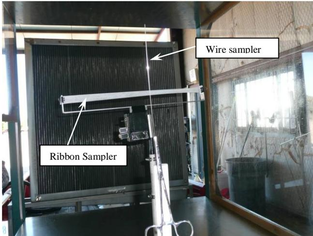
**Figure 2. View of two samplers in a wind tunnel at College Station, TX**
