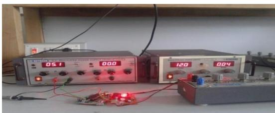
Figure (18) Hardware circuit of open loop buck converter
