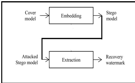
Figure 1 watermarking scheme model
